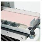
A top-loading paper feed system allows continuous operation.
