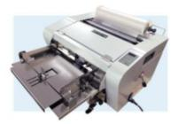
High capacity auto-feed eliminates need to insert one at a time.
