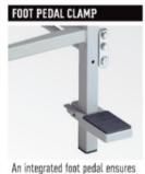
An integrated foot pedal ensures positive clamping.
